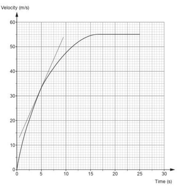
Acceleration can be calculated by measuring the gradient of a velocity-time graph.
